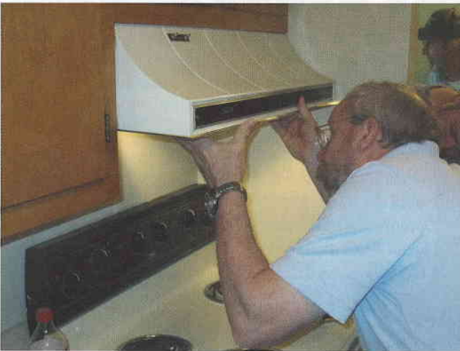
Range hood airflow verification with duct tester.
